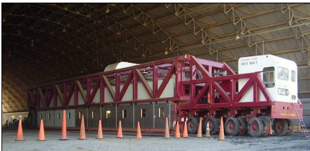
Figure 1: USCoE Heavy Vehicle Simulator at ERDC, Vicksburg, USA
